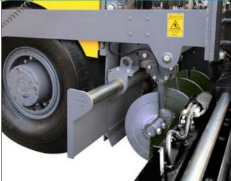
flexibility in variety of job site conditions. The speed of the conveyors are automatically adjusted independent of augers with individual ultrasonic sensors and pile height knobs for each side.
