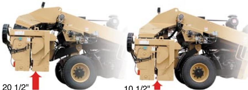
**Variable height front hopper.** Raise and lower hopper to clear obstacles. Easier loading.
